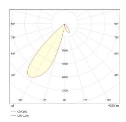
32 LED System perform. [W] Bulb type Luminous flux [lm] 4250 Current sec. [mA] 800 Colour temp. [K] 4000K CRI HE>90
